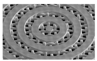
Sharp edged 80 µm circle line exposed on SEFAR® PME 140/355-30Y
