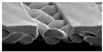
SEFAR® PET 1500 180/460-27Y, 15 μm capillary film, 7 μm EOM
