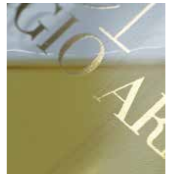
High dense sharp edged letters on perfume flacon with SEFAR® PCF FC 120/305-34Y
