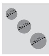
Thread diameter nominal  $d_{nom}$  [µm] The diameter  $d_{nom}$  is measured on the thread before weaving.
