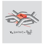
Theoretical ink volume  $V_{th}$  [cm<sup>3</sup>/m<sup>2</sup>] The theoretical ink volume  $V_{th}$  is calculated from the mesh thickness **D** and the percentage of open area  $\alpha_0$ .
