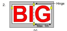
Make a hinge perpendicular to the largest dimension of the letters or logo, no more than 1m away from any one of the edges.
