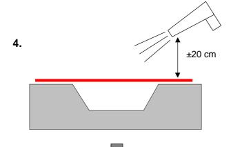
Heat MACfleet 6500 with an industrial air gun (air temperature: ±250°C).
