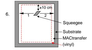
Squeegee horizontally, working from the centre outwards to the left and then the right stopping ±10 cm from the top edge of the vinyl.
