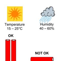
Also avoid directly exposing the vinyl to high temperatures (near radiators, in direct sunlight, etc.)
