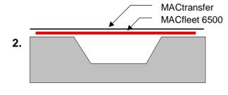
Apply MACfleet 6500 using MACtransfer application tape over the 3 dimensional surface.
