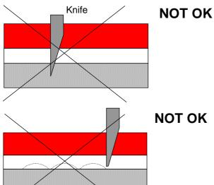
If cuts are too deep, then the backing could split when the letters or logos are being transferred onto the MACtransfer tape.
