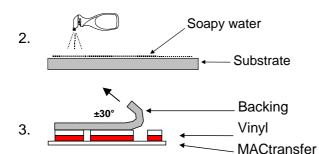
Use the spray bottle to wet the entire substrate surface (do not use a sponge or a cloth as these can leave dust, fluff, etc.).
