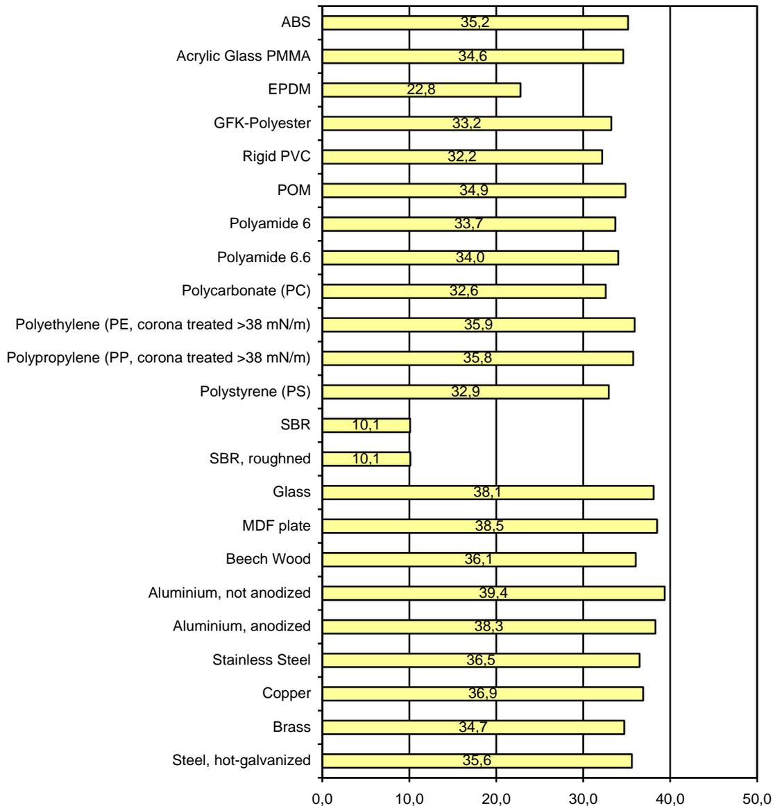
Peel strength measured as per PSTC 1 with peel tester type L 500 of Lloyd Instruments, load cell 100 N, class 1, DIN EN ISO 7500-1 for tension and pressure, 180° peel test, printed over a mesh of 21-140 (T) onto 125 µm polycarbonate film, measured after 72 hours stored in normal climate (according to DIN 50014-23/50-1), stated in N/inch. Peel speed 300 mm/min. Adhered with hand roller (according to PSTC standard, roll weight 10 pounds, rolled 5 x in each direction). Adhering area 2,5 x 10 cm.
