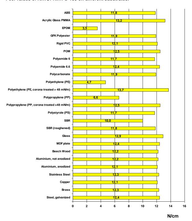
Tested according to PSTC 1. Measured with peel tester type L 500 from Lloyd Instruments. Load cell 100 N, class 1, DIN EN ISO 7500-1 for tension and pressure, peel angle: 180°, printed with 21-140(T) on 125  $\mu$ m polycarbonate film, measured after 72 h-storage at normal climate (according DIN 50014-23/50-1). Peel speed 300 mm/min. Applied with a hand roller (according to PSTC standard: 10 pounds, rolled 5x in each direction). Adhesion area: 2,5 x 10 cm. N/inch.
