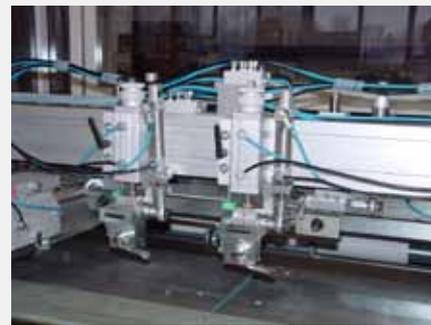
Pic.20: Anti-drip device with tilting cylinders
