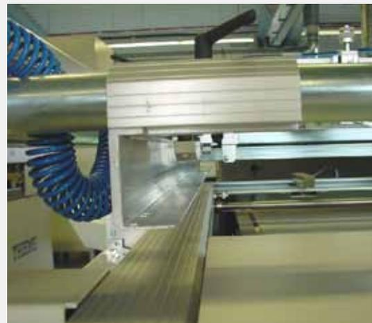
The frame is pneumatically clamped and opened. The feeding at 3 points guarantees an exact frame positioning which is absolutely required for the use of a register system! The precise screen fine tuning is made by three micrometer spindles and ranges between +/- 10 mm. The master frame is guided on balls to achieve a vibration-free screen adjustment.
