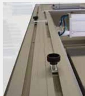
To adjust the squeegee travel, small magnetic bars situated on the top side of the guiding bar are moved and fixed by help of knurled screws.
