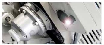
Crop mark detection. High resolution camera for crop mark detection
