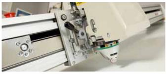
The Machine is equipped with a Plug & Play Interchangeable Head system. Powerful magnets allow to quickly hold cutting tools and work without any interruption or tools setup.
