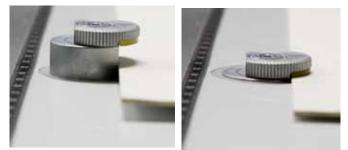
The button clamp system allows to trim the material right to the edges, optimizing the material yield.
