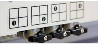
Vacuum table. Extremely reliable rotary vane vacuum pump (oil-free and air-cooled) working through a selection of four independent work areas.
